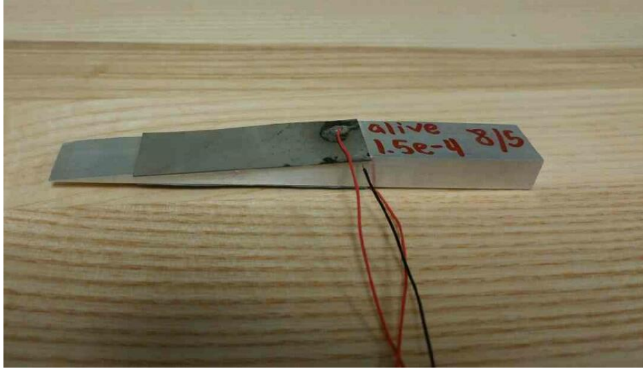
Figure 2.6: Image of a bimorph piezoelectric actuator.
